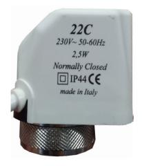
The WHS-S-230AC & WHS-S-24AC actuators have a wax thermostatic element mounted in the actuators and are activated by a thermistor against a signal send from the thermostat.
