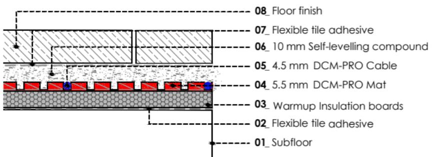
\* This method can be used to create a finished floor surface suitable for most floor finishes. When forming a drainage slope within a Wetroom installation, ensure the minimum 10mm thickness of the levelling compound is maintained in the heated areas.
