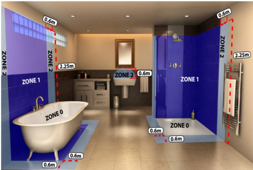
**NOTE:** In the case of bathroom installations, electrical regulations prohibit the installation of Mains Voltage products such as thermostats, contactors, fused spurs, isolators or junction boxes, within Zones 0 or 1.
