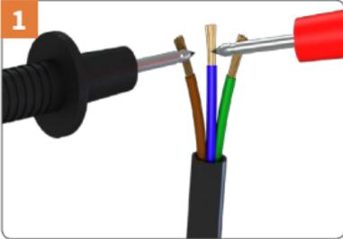
When the tiles or levelling compound has been installed, conduct another resistance test as described on Page 28 to ensure the sensor and heater have not been damaged and record in the control card on Page 30.
