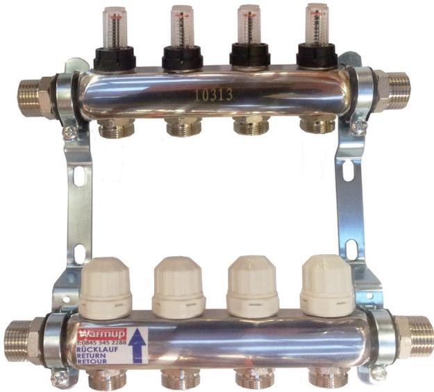
The Warmup Steel Range of manifolds are available from 2 to 12 circuits, sized to the requirements of the project. Most systems are operated at 1 bar pressure, however at Warmup our manifolds are pressure tested to 10 bar at the manufacturing stage to ensure that the highest quality is maintained.
