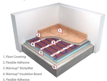
The Warmup StickyMat underfloor heating system is suitable for all projects: new build, retrofits and refurbishments.
