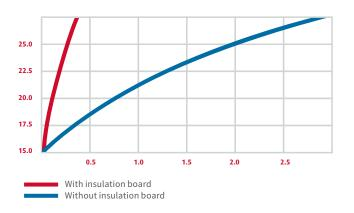
The Warmup Research Centre found that response times were cut from over 2.5 hours to just 20 minutes by including Warmup Coated Insulation within the system installation, placing it between the Warmup Electric Underfloor Heating System and the concrete sub floor.
